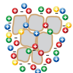
Coating of humate provides charged surface to hold nutrients
